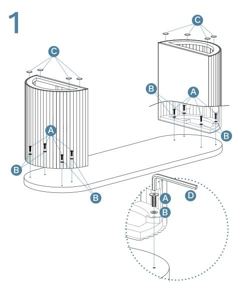
Attach 2x bases to the top panel with 8x bolts (A) and 8x flat washer (B). Tighten all bolts with allen key (D). Attach 8x foot pads (C) to the bottom of the base.
